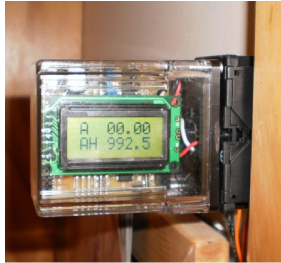
Photo-3 : Amp-Hour meter (T690 module)
